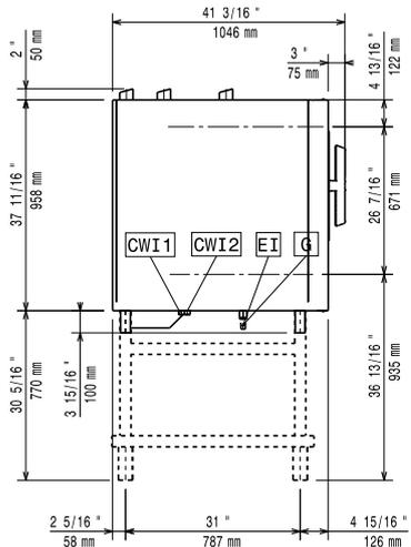
CWI1 = Cold Water inlet 1 (cleaning)      EI = Electrical inlet (power)
